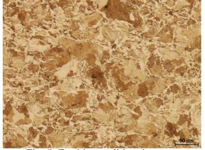
Fig. 5. Ferritic-pearlitic microstructure of the specimen made of 30MnB4 steel after a deformation cycle cooled with the rate of  $5^{\circ}C/s$
