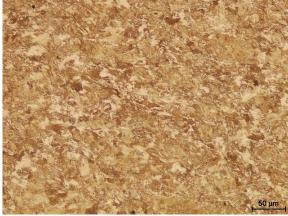
Fig. 6. Ferritic-pearlitic microstructure of the specimen made of 30MnB4 steel after a deformation cycle cooled with the rate of 10°C/s
