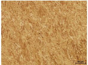
Fig. 7. Martensitic-bainitic microstructure of the specimen made of 30MnB4 steel after a deformation cycle cooled with the rate of 80°C/s
